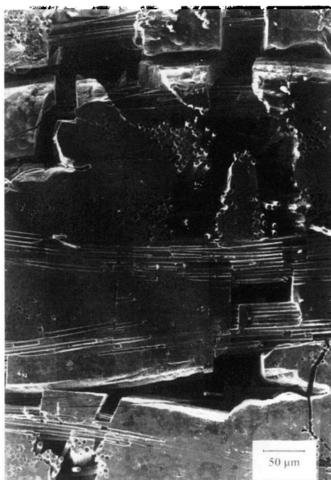
Figure 3. SEM micrograph of a 2D \text{SiC}_f -SiC specimen creep tested in tension, until rupture, under argon, at 1373 K, under 125 MPa.
